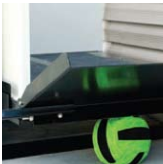
Safety sensors stop lift if obstacles encountered
